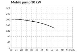
$m^{\scriptscriptstyle 3}/h$  - capacity /  $\,m$  - height of water elevation
